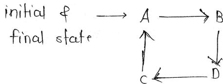
$$\left. \begin{aligned} &\text{change in state function for cyclic process} = 0 \\ &\Delta U = \Delta H = \Delta G = \Delta S = 0 = \Delta A \\ &\oint dU = 0 \qquad \oint dH = 0 \end{aligned} \right\}$$
