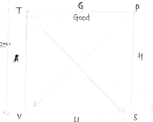
$$\left(\frac{\partial T}{\partial V}\right)_S = - \left(\frac{\partial P}{\partial S}\right)_V$$
