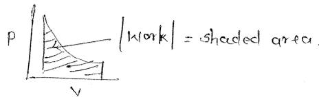
$$W = - \int_{V_1}^{V_2} P dV. \quad \text{--- isothermal irreversible process}$$
