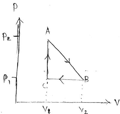
$$\begin{aligned} \text{net work done} &= \text{Area of triangle} \\ &= \frac{1}{2} \text{base} \times \text{height} \\ &= \frac{1}{2} (V_2 - V_1) (P_2 - P_1) \end{aligned}$$
