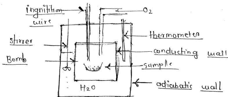
Bomb calorimeter. ( $\Delta U$ ) calculation.
