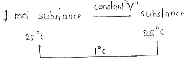
$q_V = C_V$  — {  $q$  required to raise the temp. of 1 mole of substance by 1°C at constant volume. }
